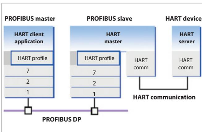
Figure 11: HART on PROFIBUS communication.
