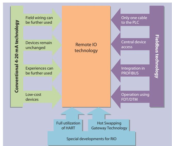
Figure 6: Attractive technology mix for remote I/O.
