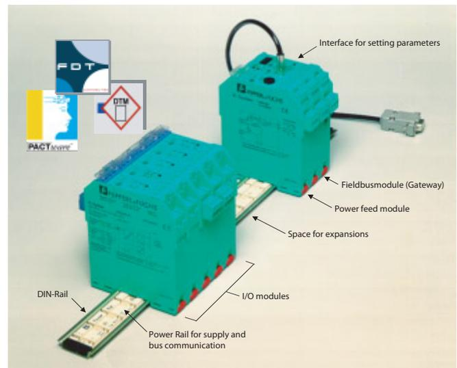
Figure 5: Modular structure of a Remote I/O system based on the example of RPI.
